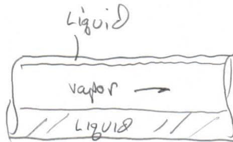
$$h_{\text{internal horiz}} = 0.555 \left[ \frac{g \rho_L (\rho_L - \rho_V) k_L^3}{\mu_L (T_{\text{sat}} - T_s) D} \left( h_{fg} + \frac{3}{8} C_{p,L} (T_{\text{sat}} - T_s) \right) \right]^{1/4}$$
