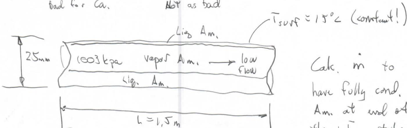
Calc. in to have fully cond. Am. at end of the 1.5 m tube,  $Re_{\text{vapor}} < 35,000$  (verify this)
